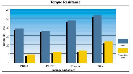
High mechanical strength helps keep heat sinks where they are supposed to be.
